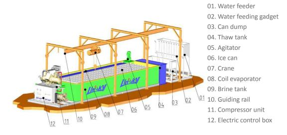
\* The diagram of brine system block ice machine working principle
